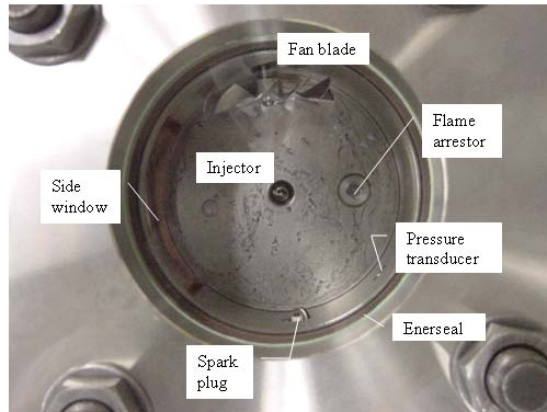
Figure 3. View of combustion chamber from the top of the end window.
